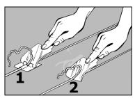
CAUTION: Welded seams must cool to room temperature before trimming. Start trimming where you began welding. All trimming of welding thread is recommended in two steps: rough and fine trimming.
