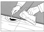
Fold back and loosen the sheets covering half of the floor area. Apply the adhesive on the subfloor with a fine-notched trowel. Use a soft brush around drains and hard-to-reach areas. Around and inside drains, please see drain manufacturers recommendation.
