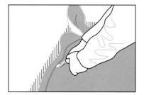
Avoid sharp creasing tools. When coving we highly recommend to use a Tarkett Hockey Stick or a Tarkett Corner Roller to press the material firmly into the juncture between the floor and wall. In areas where one sheet is sufficient to cover the subfloor, the adhesive can be applied over the entire surface area before installing the sheet. Although this requires experience, it is the fastest installation method.
