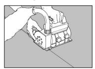
The sheets are hot welded. Do not weld until the adhesive has bonded completely, wait 24-48h. The joints are chamfered or grooved to about ¾ of the thickness using a hand grooving tool or machine prior to welding.
