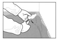
When fitting in-corners, make a cut in the excess material starting about 5 mm (about ¼ in.) above the floor in the corner. If the material has to be heated before folding, heat the area between the sheet and the wall. This provides better contact between the sheet and adhesive.
