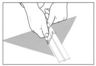
To glue the triangle-shaped piece more simply and securely, cut a groove on the back of the triangle with Tarkett Corner Knife. The depth of the groove shall be no deeper than half of the sheet thickness.
