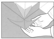
The triangle can now be folded and placed on the corner. It will overlap the coved floor. Cut through the overlapping material to make a tight fit.
