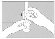
2) Prefabricated covers are applied according to the manufacturer's instructions. Seam sealer or sealing compound approved for this purpose, can be used for an extra tight fit around pipes.
